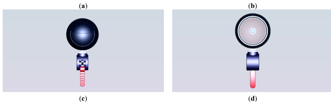
Fig. 4. Design of the light lamp in circular shapes using the light source and reducing the cost of producing reflective mirrors. Heat dissipation holes are not found. (a) oblique front view, (b) side view, (c) rear frontal view, and (d) frontal view.
