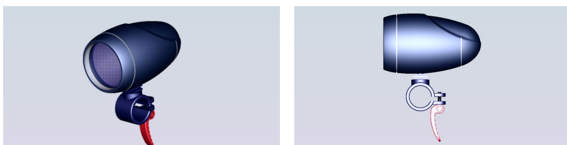
Fig. 3. Design of the light lamp in circular shapes using the light source and reducing the cost of producing reflective mirrors. Heat dissipation holes are found in figures. (a) oblique front view, (b) side view, (c) rear frontal view, and (d) bottom view.
