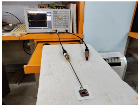
Fig. 11. Experiment setup of measured resonant frequency of NFC tag.
