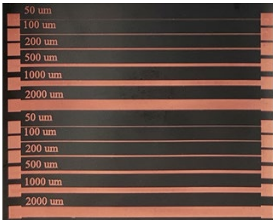
Fig. 6. Photograph of chemical copper plated contrast pattern of Ni-Zn-Cu ferrite.
