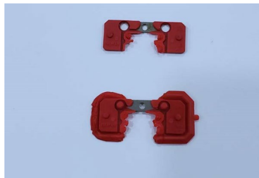
Fig. 2. Rail block defects
